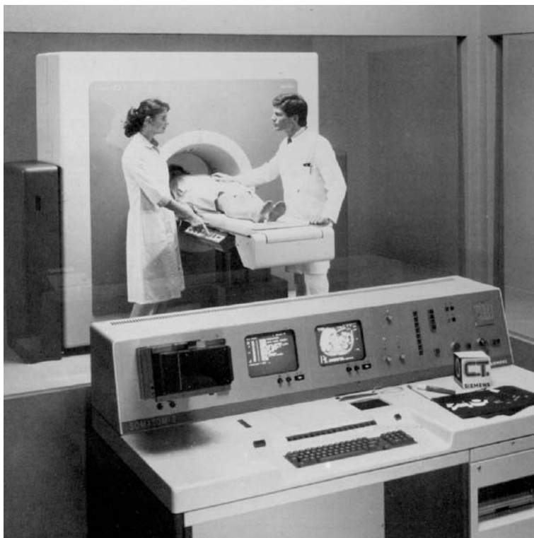
Fig. 3.11. An example of a whole body scanner from 1981: The Siemens Somatom family DR. This third generation of computed tomography scanners has a measuring field of approximately 53 cm in diameter. With 512 solid state detectors, acquisition times of about 3 s were possible for a 360° rotation (courtesy of Siemens Medical Solutions)
