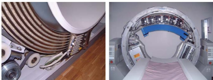
Fig. 3.15. Different methods of energy transfer to the continuously rotating sampling unit. In the Siemens Somatom AR.T ( left ), slip-ring technology is used. In the compact mobile CT scanner of the Philips Tomoscan M ( right ) an accumulator array is used
